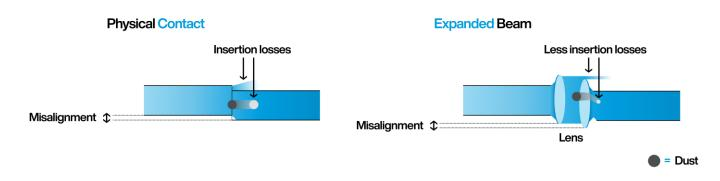
Contamination is a recurring problem faced by physical contact connectors, where a focused beam is subject to signal losses due to microscopic debris.
